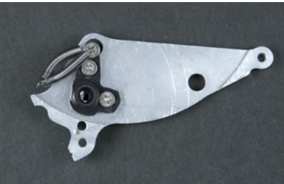
Figure 8-45. Kicker leg with servo horn attached
