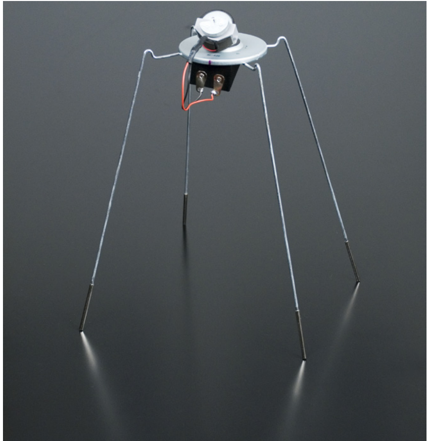
Figure 3-21. Vibrating robot, still lacking the ultrasonic sensor
