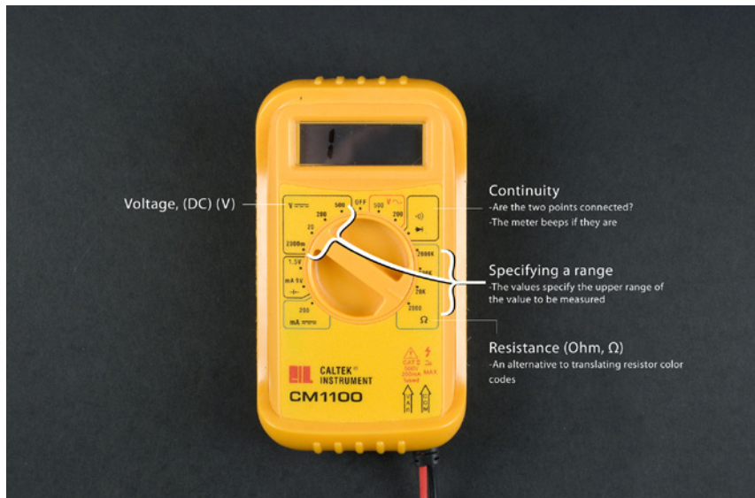
Figure 1-26. The most common functions of a multimeter
