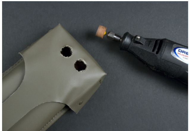
Figure 3-27. Holes created with a mini drill
