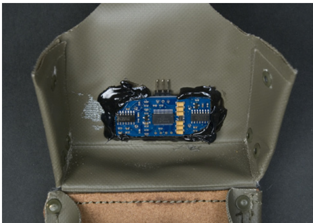
Figure 3-28. A hot-glued ultrasonic sensor
