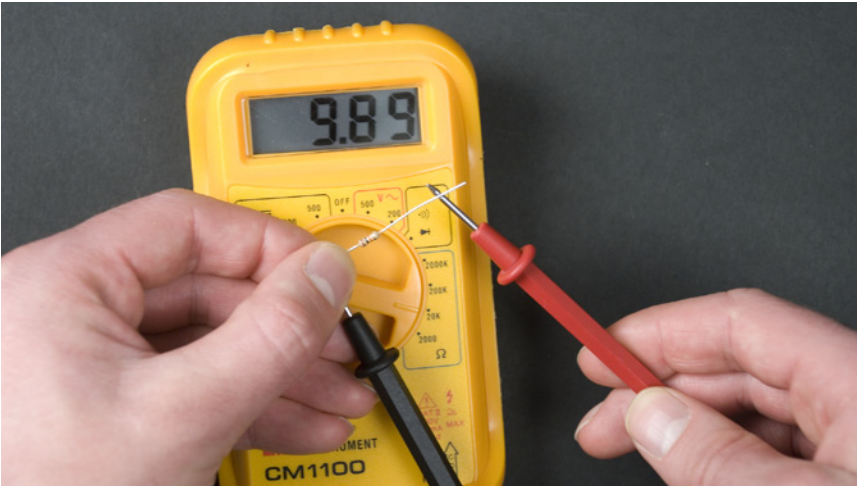
Figure 5-6. Measuring resistance with a multimeter
