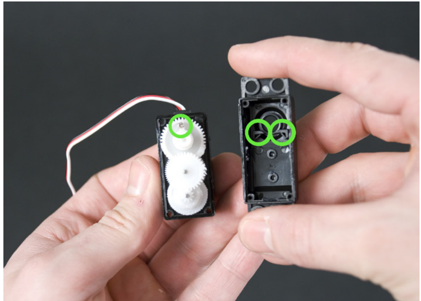
Figure 8-9. Obstructions that block rotation
