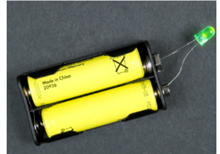
Figure 1-28. Simple closed circuit powering an LED
