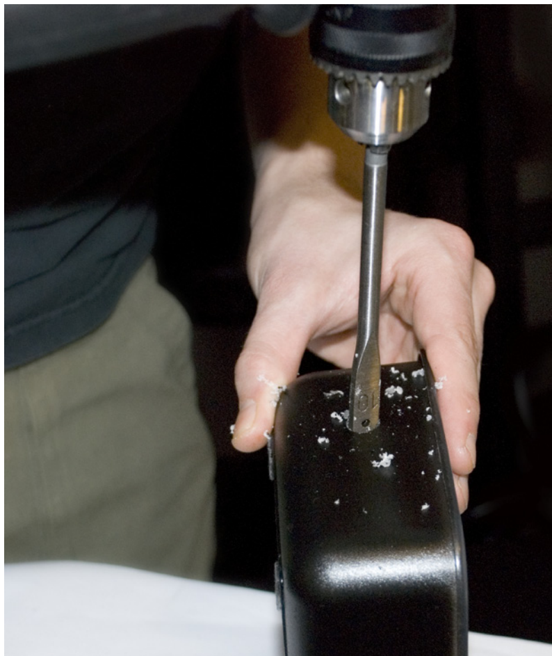
Figure 7-33. Drilling a hole for the USB cable
