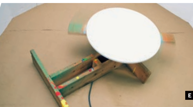
Fig. A: Corded drill mounted on the wooden base. Fig. B: To make an adapter that holds the canvases, hammer a T-nut into the center of a 1×4, screw a bolt through the T-nut, and chuck the bolt into the drill.
