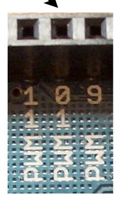
The PWM speed used for analogWrite() is set to 450Hz or 30 kHz currently. I forget which, but it's not something changeable without understanding more about how AVRs work. So when programming AVRs in C outside of Arduino, PWM speed can be set to just about any value.
