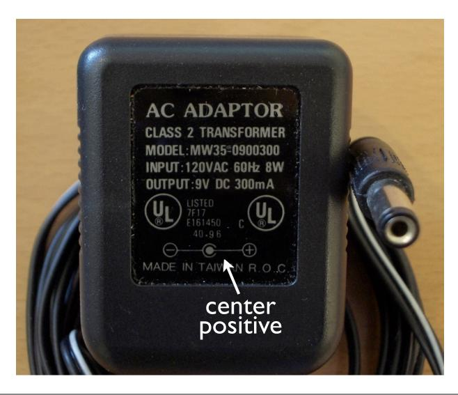
Actually input voltage can be from like 7.5V to 35V, but don't go over 15V so the voltage regulator doesn't have to work so hard.
