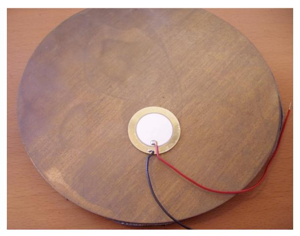
Here's one glued to a larger brass disc for a drum trigger
