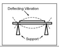
Oscillating voltage alternately squeezes and releases the piezo element. Must apply flucuating voltage, a steady HIGH or LOW won't work.
