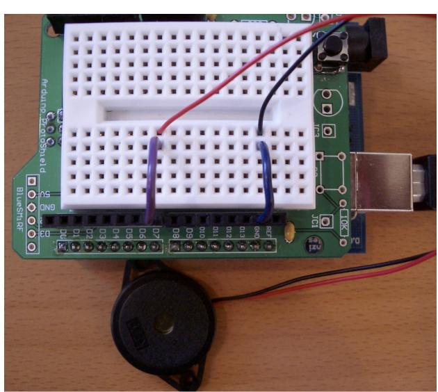
Piezo leads are very thin. The breadboard holes grab them better than the header sockets, which is why the jumper leads are used.
