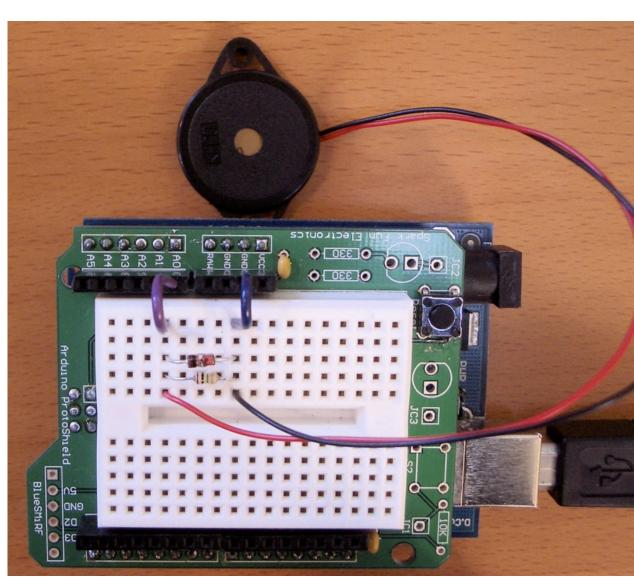
Create two little busses for GND and A0, and hook components across it. Black bar on diode indicates "bar" of diode.
