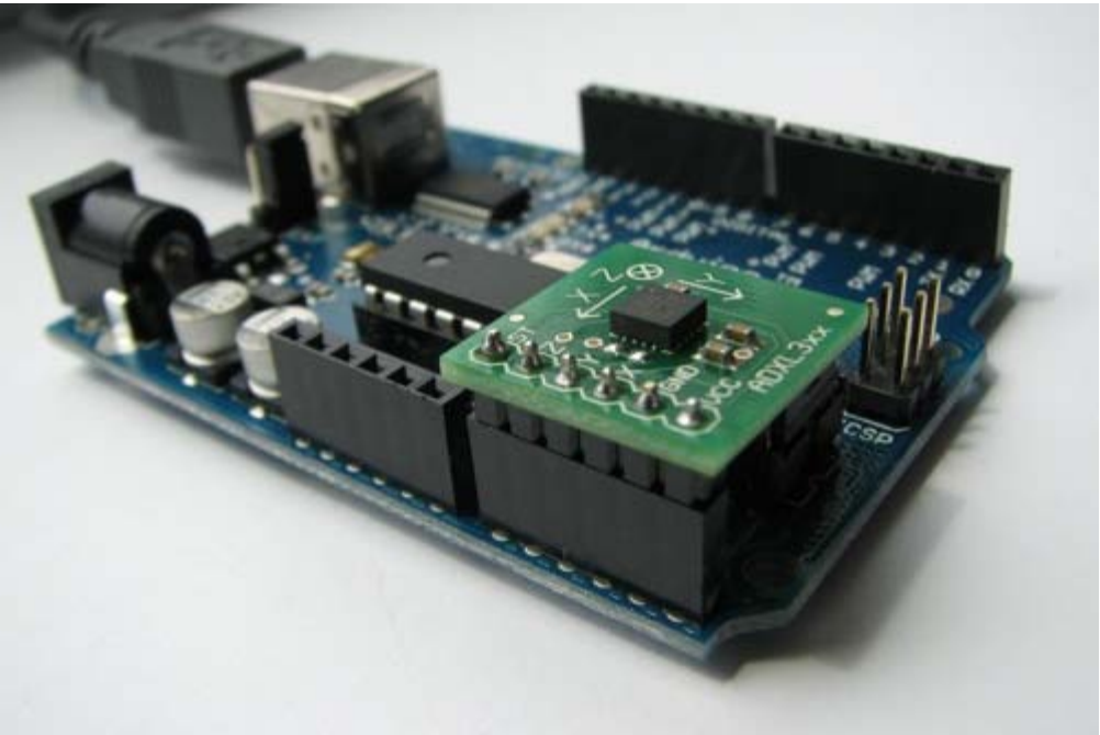
An ADXL322 on a Sparkfun breakout board inserted into the analog input pins of an Arduino.
